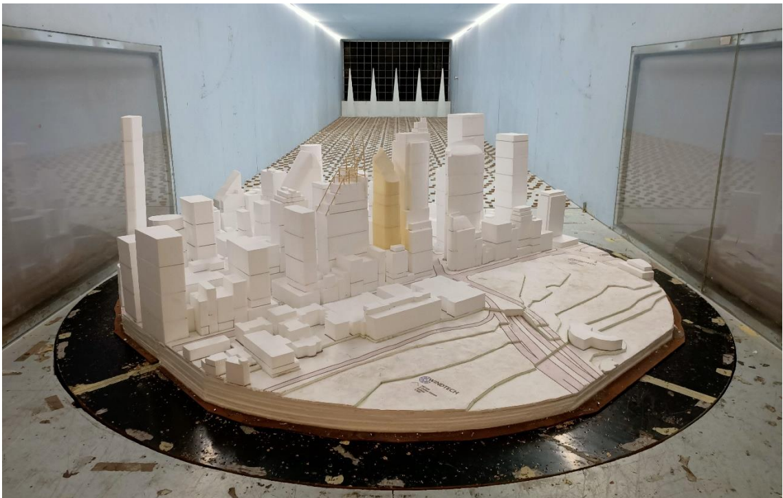
Figure 1c: Photograph of the Wind Tunnel Model (Base Case, view from the south-east)
